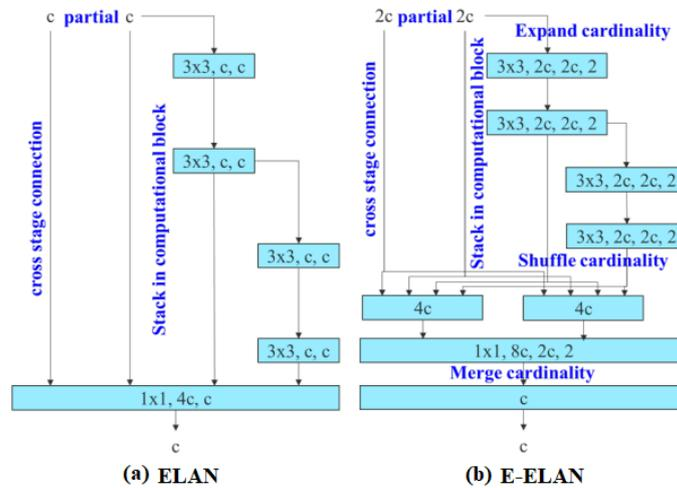
Figure 2. ELAN and E-ELAN architectures ((Wang et al. 2022))
