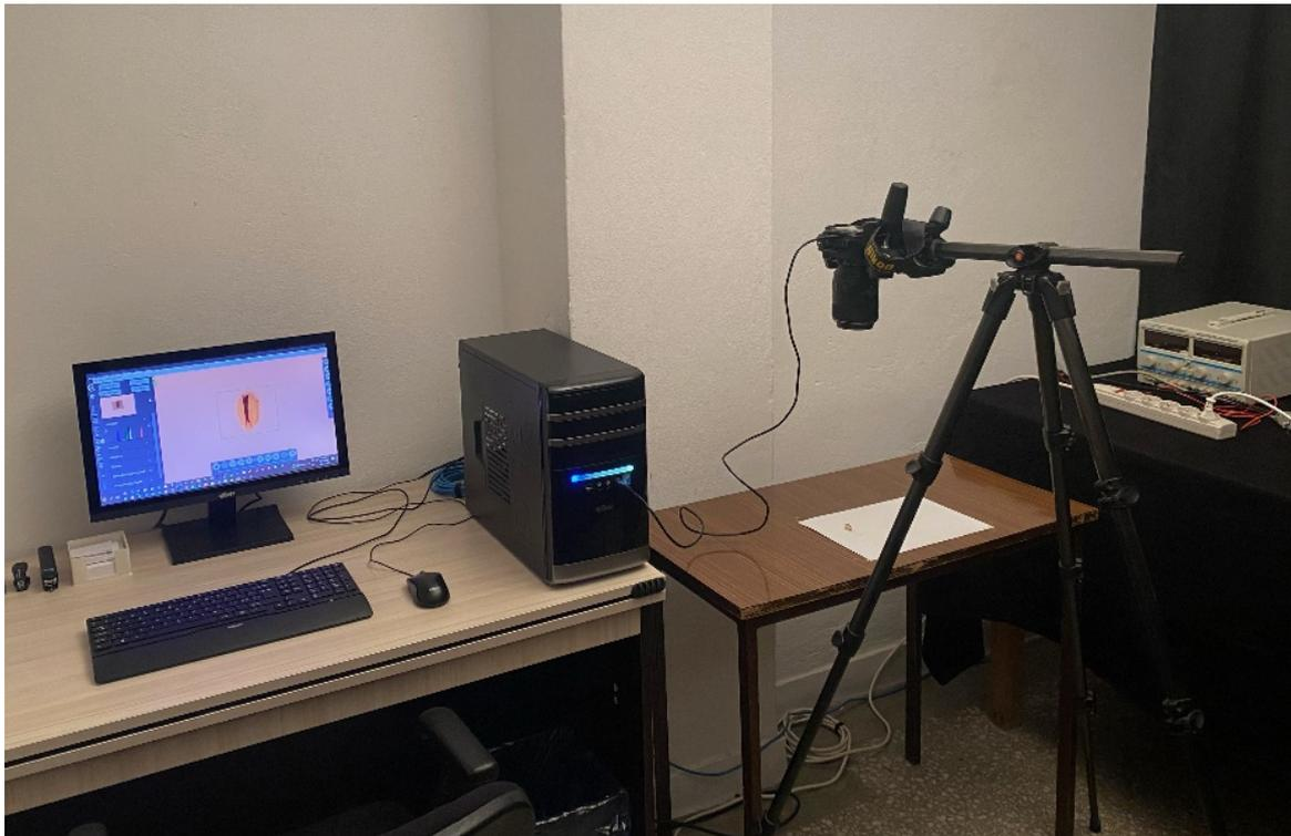
Figure 2. Antep pistachio nuts image capture set-up.
