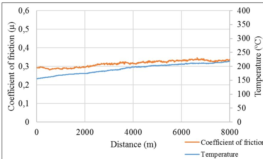
Figure 10. 35 MPa friction coefficient and temperature graph.
