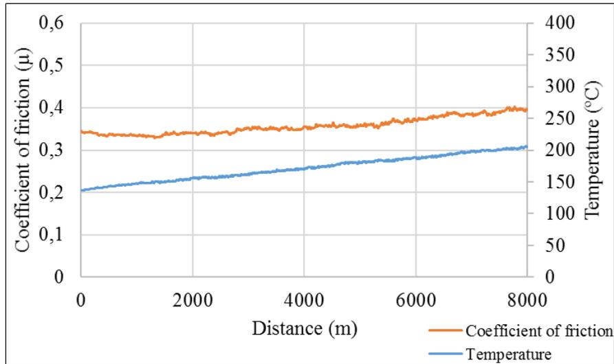
Figure 11. 40 MPa friction coefficient and temperature graph.
