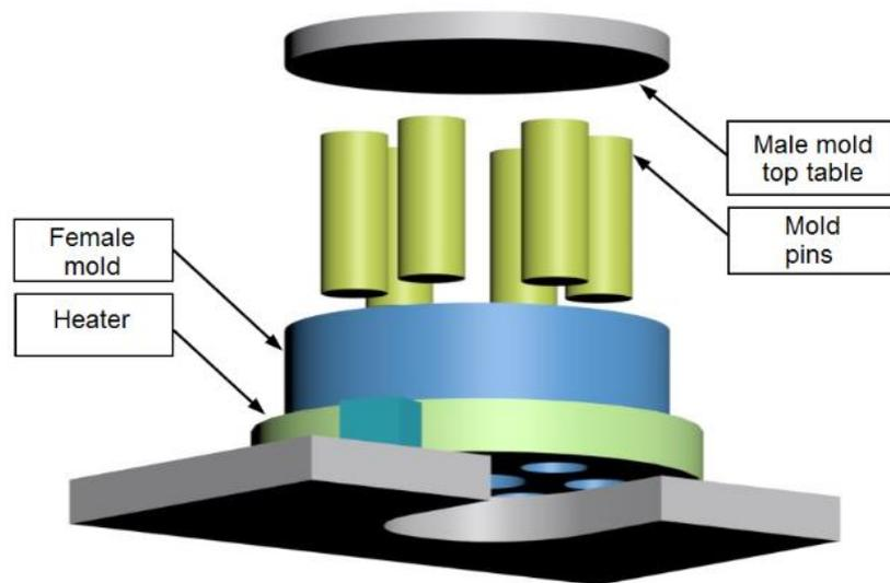
**Figure 1.** View of mold design.
