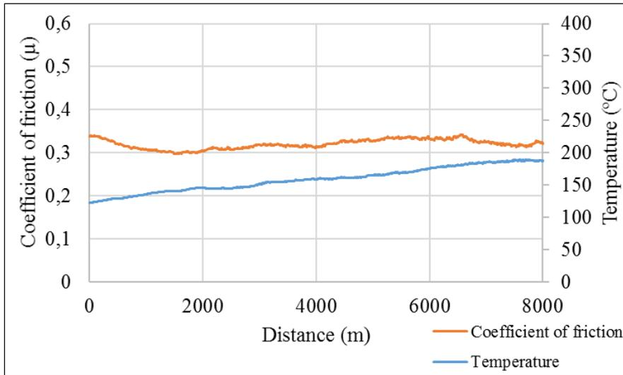
**Figure 7.** 20 MPa friction coefficient and temperature graph.
