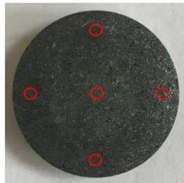
**Figure 3.** Hardness measurement points.
