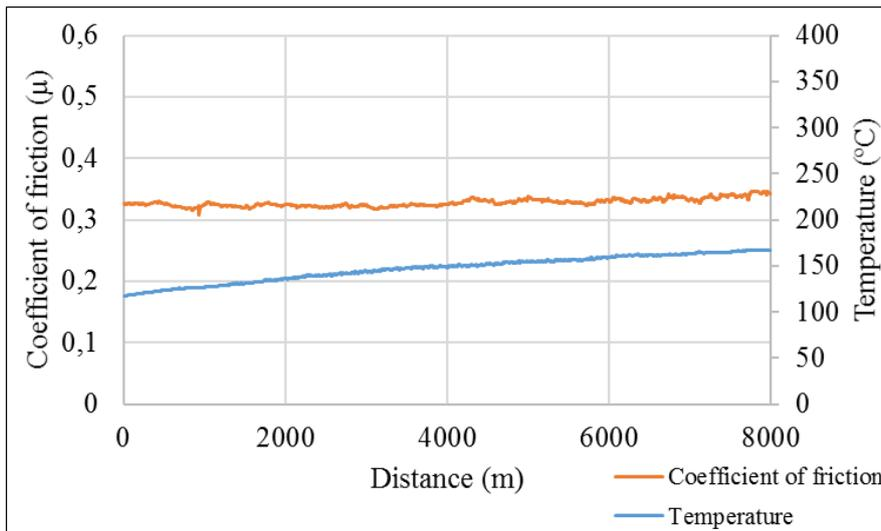
**Figure 8.** 25 MPa friction coefficient and temperature graph.
