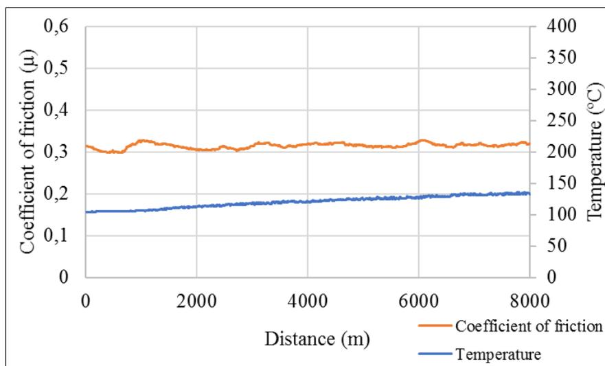
Figure 6. 15 MPa friction coefficient and temperature graph.
