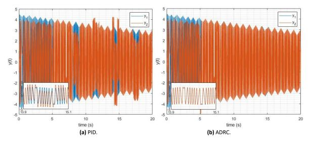
Figure 9. Synchronization of y(t) function with PID (a) and ADRC (b) under disturbance.
