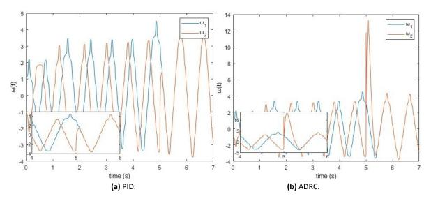
**Figure 7.** Synchronization of  $\omega(t)$  function with PID (a) and ADRC (b).
