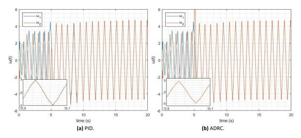
**Figure 11.** Synchronization of  $\omega(t)$  function with PID (a) and ADRC (b) under disturbance.
