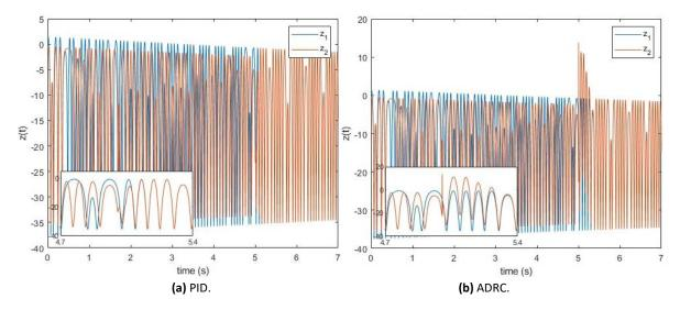
**Figure 6.** Synchronization of z(t) function with PID (a) and ADRC (b).
