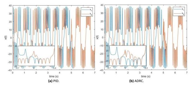
**Figure 4.** Synchronization of x(t) function with PID (a) and ADRC (b).
