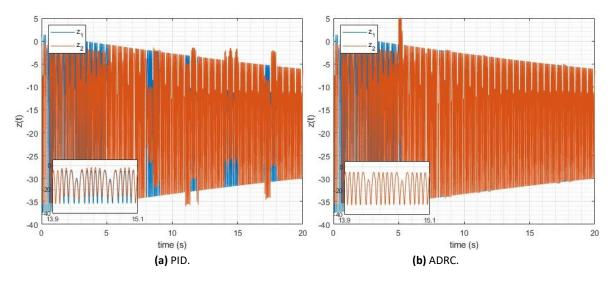
Figure 10. Synchronization of z(t) function with PID (a) and ADRC (b) under disturbance.
