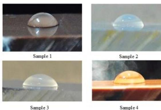
**Figure.** Contact angle measurements of Polyvinyl chloride samples
