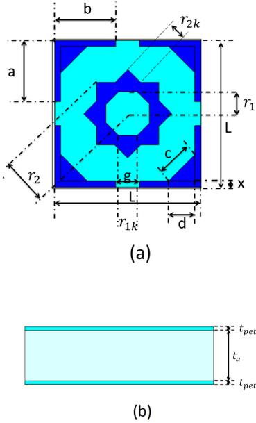
Fig. 1. (a) Front profile and (b) side profile of proposed metamaterial based transparent absorbent design
