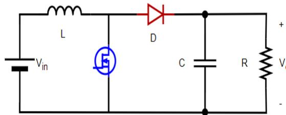
**Figure 5.** The circuit topology of boost converter
