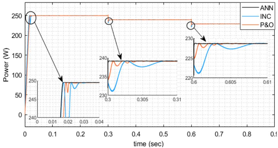
**Figure 15.** Constant irradiance and variable temperature
