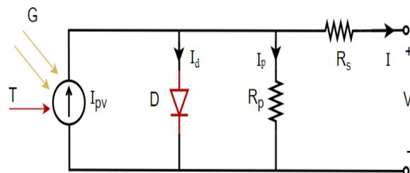
**Figure 2.** Equivalent circuit of cell with one diode
