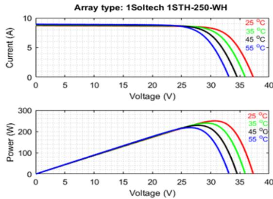
**Figure 4.** I-V and P-V curves of the PV system at constant  $1000 \text{ W/m}^2$
