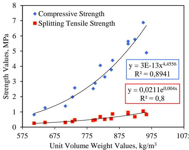
Figure 8 Strength versus Unit Volume Weight of CLCM specimens
