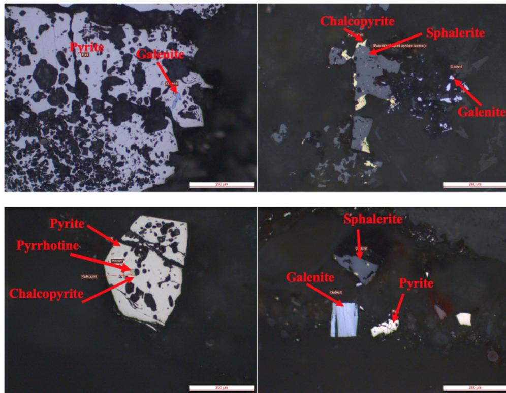
Figure 5. Polish section photos of the sample
