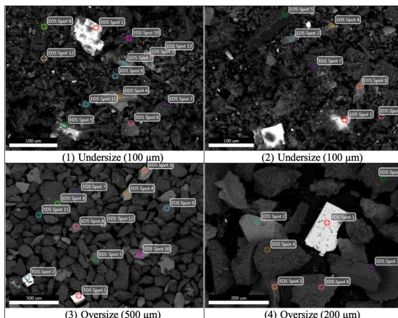
Figure 4. SEM photos of the sample subjected to EDS analysis
